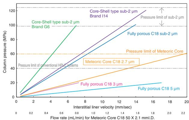
Meteoric Core C18 has high column efficiency which is almost equivalent to sub-2 μm columns over a wide range of flow rate.
