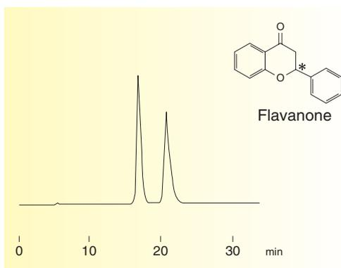
Column : YMC CHIRAL PREP CD PM (10  $\mu\text{m}$ , 120  $\text{\AA}$ )
