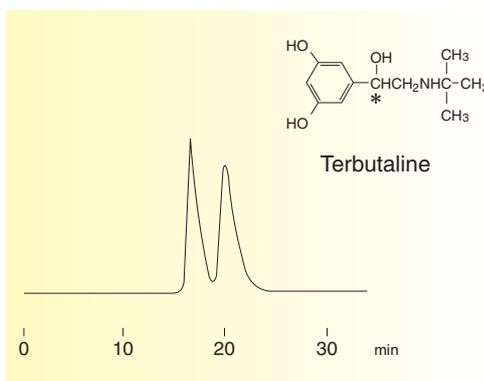
Column : YMC CHIRAL PREP CD ST (10  $\mu\text{m}$ , 120  $\text{\AA}$ )
