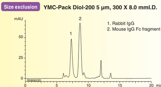
Eluent : 0.1 M  $\text{KH}_2\text{PO}_4$ - $\text{K}_2\text{HPO}_4$  (pH 6.9) containing 0.2 M NaCl
