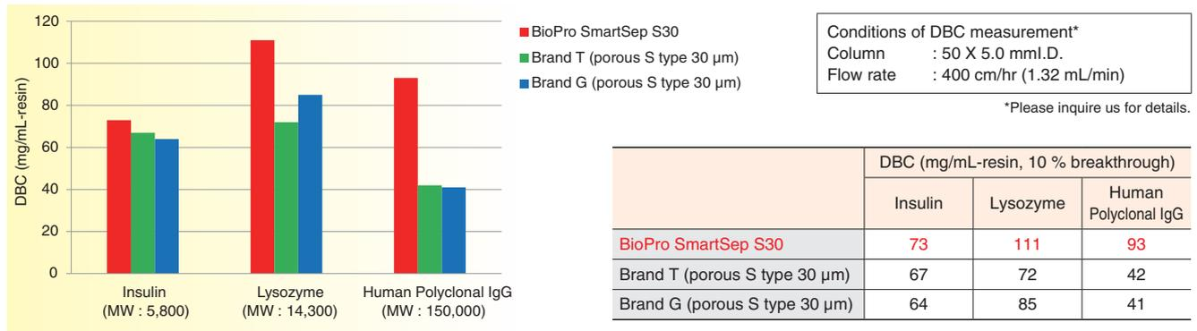
BioPro SmartSep ion exchange media have higher DBC compared to conventional ion exchange media. Especially for IgG, BioPro SmartSep has more than twice as high DBC as competitors'. This feature of BioPro SmartSep makes purification productivity of IgG per unit time double or more.
