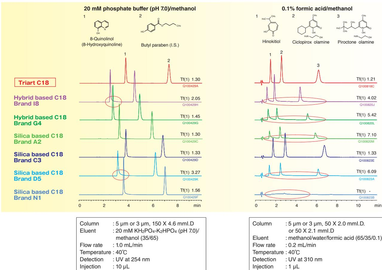
Triart C18 is able to provide excellent peak shapes for coordination compounds which are often absorbed to a column, resulting from a strong interaction with impurities such as metal ion.
