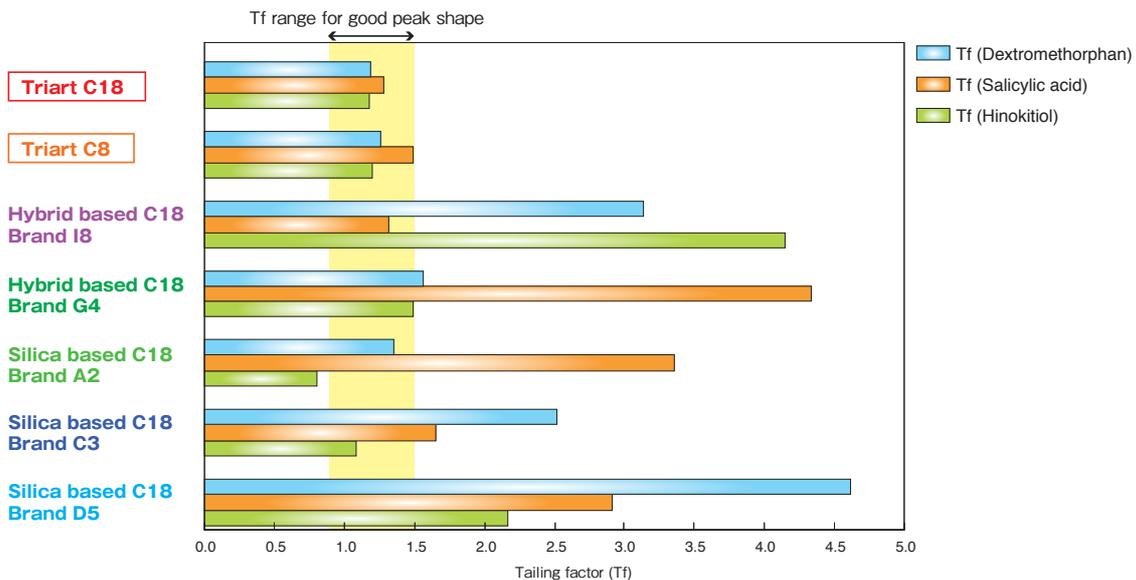
The peak tailing or fronting of ionic compounds are often caused by adsorption to residual silanol groups and/or surface impurities resulting from base materials or manufacturing process. Triart, based on hybrid silica material with little metal impurities and rigorously endcapped, provides symmetrical peak shapes for all types of compounds.
