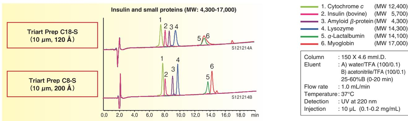
Proteins with molecular weight (MW) of 10,000 or larger are effectively separated with Triart Prep C8-S while there is little difference in separation of proteins with MW of less than 10,000 between Triart Prep C18-S and Triart Prep C8-S. It is useful to select optimal phase for establishing effective preparative method.
