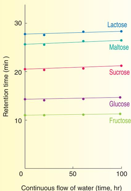
Even in a hard flow durability test using a mobile phase that consists only of water, the retention time of sugars changes little.
