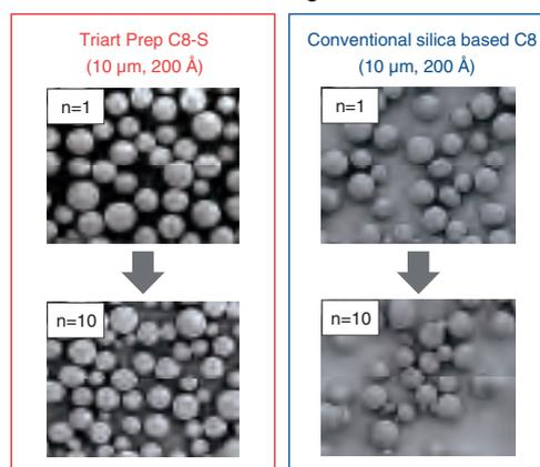
Triart Prep material still remained initial state after more than 10 times of repacking. On the other hand, conventional silica showed pressure increase or crush of particles. Triart Prep with its high mechanical stability enables longer column lifetime, and this feature provides reduction of purification cost.
