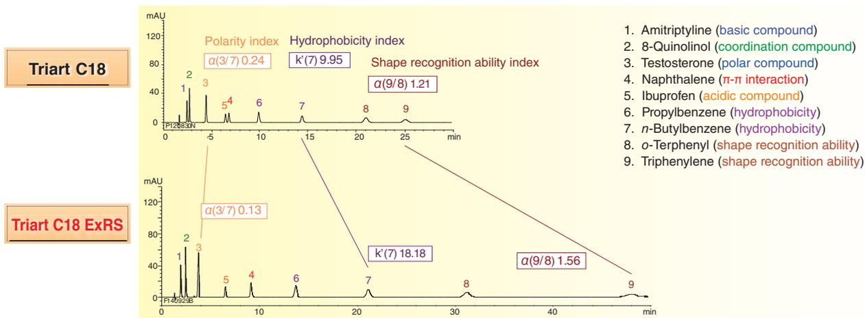
A mixture that consists of compounds with various characteristics is analyzed with Triart C18 and Triart C18 ExRS. Triart C18 ExRS has lower polarity and higher hydrophobicity than the standard Triart C18 column. It also shows improved planar cognitive ability.
