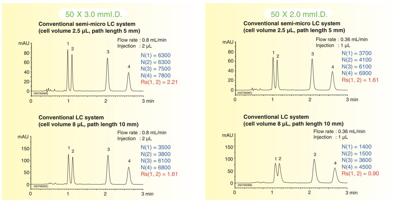
YMC-UltraHT series can be used for fast analysis with conventional LC system, as its pressure is lower than commercial sub-2  $\mu$ m columns. Considering the extra column band broadening, the column of 3.0 mmI.D. is more applicable for conventional LC system than the column of 2.0 mmI.D..
