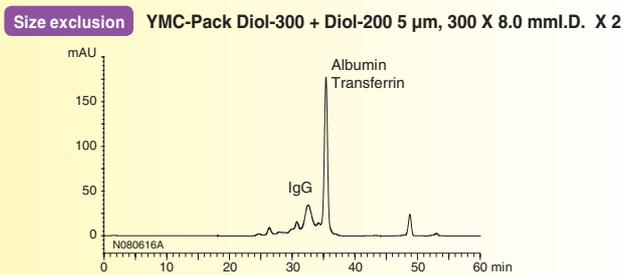
Eluent : 0.1 M  $\text{KH}_2\text{PO}_4$ - $\text{K}_2\text{HPO}_4$  (pH 7.0) containing 0.2 M NaCl
