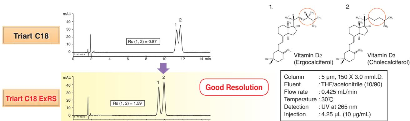
Triart C18 ExRS is effective for separating of structural analogs. This feature is especially useful for separating pharmaceuticals with structurally similar impurities
