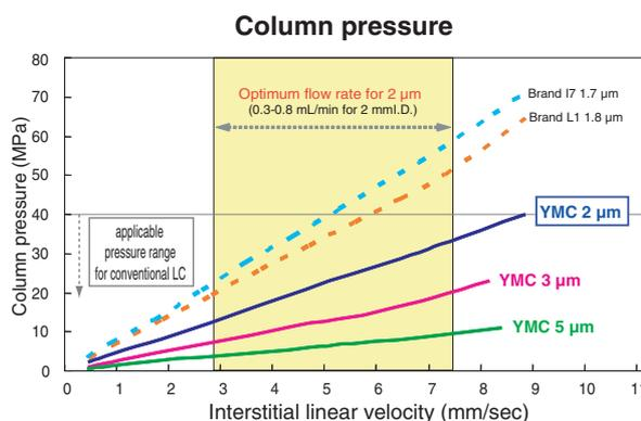
YMC-UltraHT series shows nearly the same efficiency as sub-2 µm columns for ultra fast LC system and reduces the column pressure significantly.
