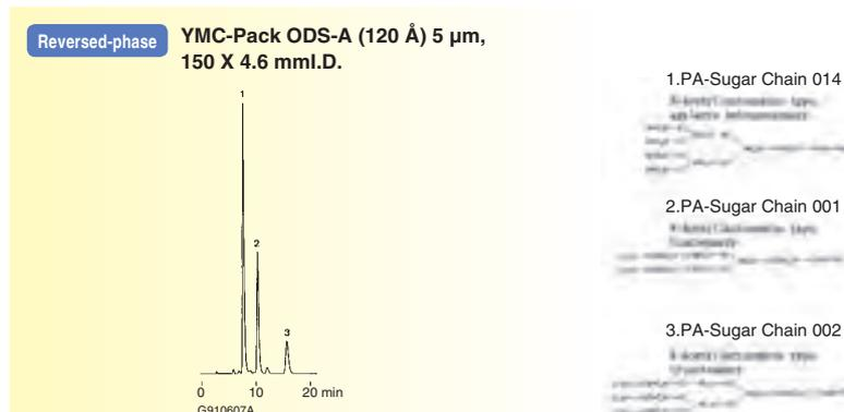
Eluent : methanol/20 mM NH<sub>4</sub>H<sub>2</sub>PO<sub>4</sub> (5/95)
