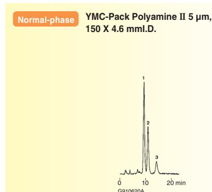
Eluent : methanol/20 mM NH<sub>4</sub>H<sub>2</sub>PO<sub>4</sub> (80/20)
