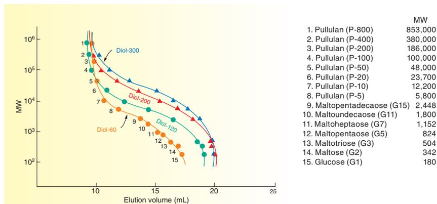
For separation or molecular weight determination of water-soluble oligo- and polysaccharides, Diol-60, Diol-120, Diol-200, and Diol-300 are useful individually or in combination.
