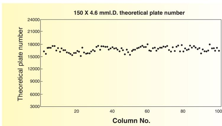
Advanced packing technology results in high column efficiency. All packed columns are inspected and controlled according to the strictest quality control criteria for column performance ever, including theoretical plate number testing.
