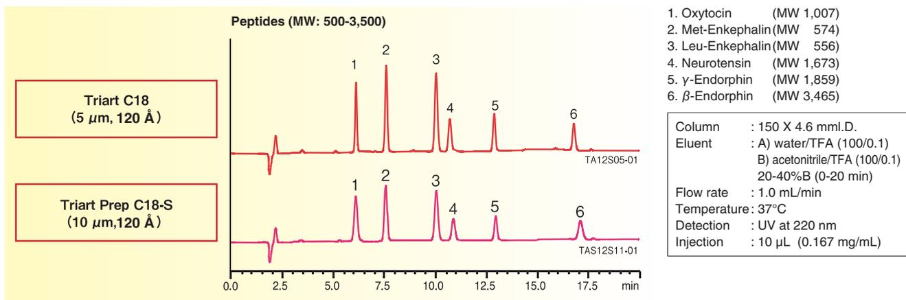
Triart Prep C18-S has identical selectivity to analytical Triart C18. A method established with analytical Triart C18 can be directly transferred to preparative scale with Triart Prep C18-S material.
