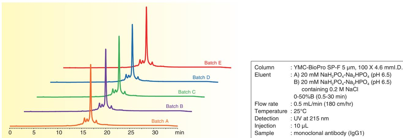
YMC-BioPro SP-F column exhibits excellent batch-to-batch reproducibility on MAb analysis, and even on resolution of peaks for small charge variants. All the gel batches are inspected by various quality control tests including HPLC analysis of MAb, and must pass rigorous criteria before release. YMC-BioPro ion exchange columns are the best choice for the quality control of MAb and other biopharmaceuticals.
