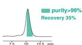
In analytical scale, many impurities could be separated from the target compound by onenucleotide difference on Hydrosphere C18. Even in purification scale, YMC-Actus gave superior separation and recovery. YMC-Actus Hydrosphere C18 is useful for purification of hydrophilic compounds such as oligonucleotides, organic acids, oligosaccharides and glycosides.
