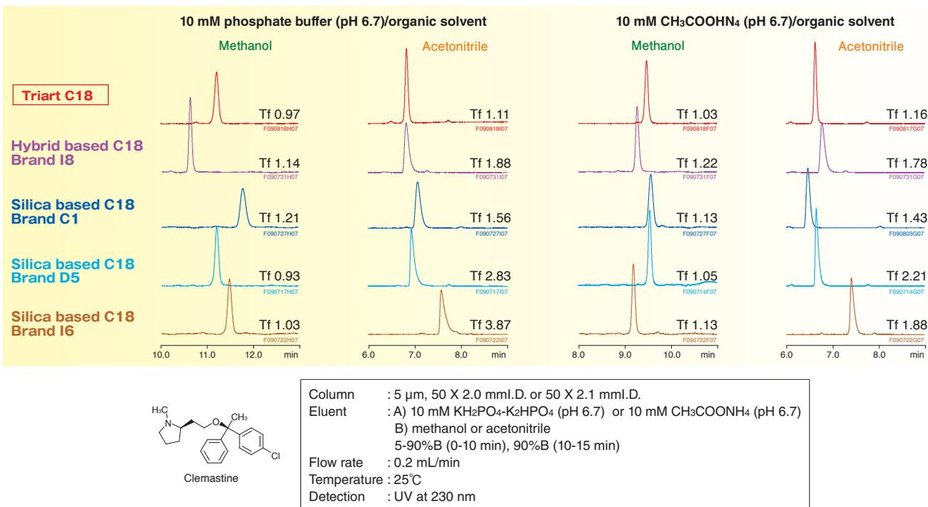
Clemastine is a well known basic compound which can easily tail on conventional ODS columns. Triart C18 can analyze clemastine without any peak deterioration with any kinds of buffer/solvent combinations.
