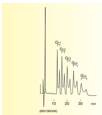
This product is useful for separations using mobile phases in which water content is relatively high, such as separation of sugars and glycosides.
