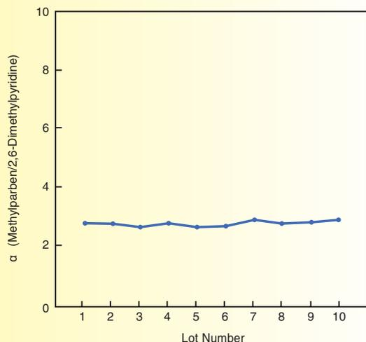
The separation factor ( $\alpha$ ) of methylparaben/2,6-dimethylpyridine for 10 lots of ODS-AM packing material is plotted on the left graph. Excellent lot-to-lot reproducibility is achieved even in separation of basic compounds.
