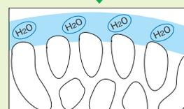
The surface of packing material is not fully hydrated. Compounds are not partitioned between mobile phase and stationary phase, and therefore its retention becomes shorter.
