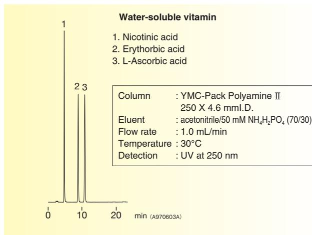
YMC-Pack Polyamine II is applicable for separation of fat-soluble vitamins and water-soluble vitamins as a normal-phase column that can be used with water or buffer and various organic solvents.
