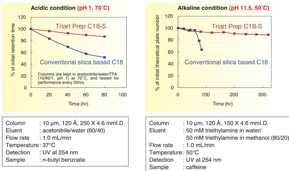
Triart Prep materials provide strong acidity-proof in the lower pH condition and alkaline-proof in the higher pH. These features enables purification with a mobile phase containing TFA and cleaning with alkaline solution, which are often used on peptides and proteins purification.
