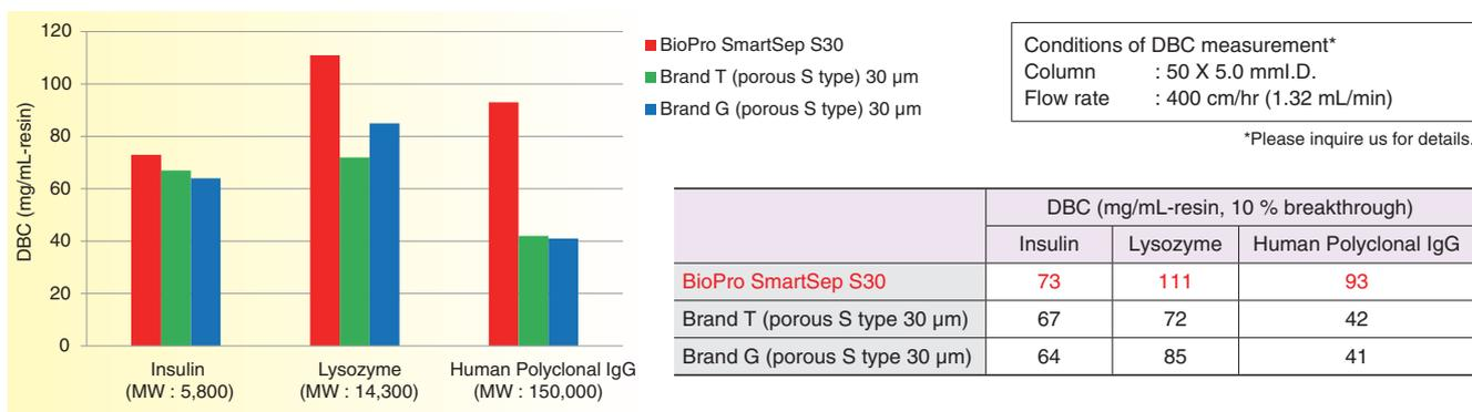
BioPro SmartSep ion exchange media have higher DBC compared to conventional ion exchange media. Especially for IgG, BioPro SmartSep has more than twice as high DBC as competitors'. This feature of BioPro SmartSep makes purification productivity of IgG per unit time double or more.
