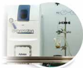
Compound identification by direct injection
