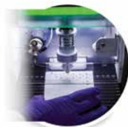
TLC/CMS – mass analysis of TLC spots
